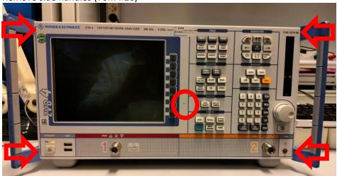
Remove the small cross screw in the middle of front panel. The remove carefully the front panel.
